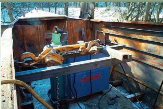
When the framework is in the right place a steel eye is welded onto the inside of the hull (just above the frame). The winch is then attached to the eye at one side and to the framework at the other.
