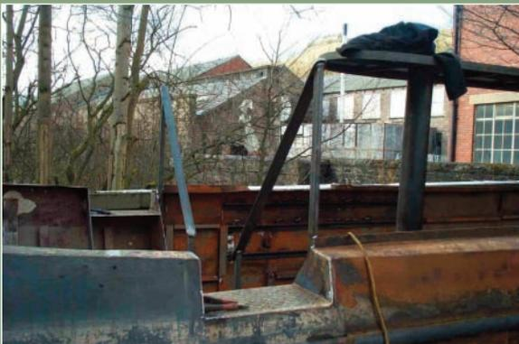
Two sturdy new T studs are welded onto the front of the boat. This is necessary as we don't want passengers clambering all over the front of the boat to get to the original T stud.
