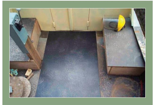
The bench seating is attached to the metal framework constructed in the front of the boat.
