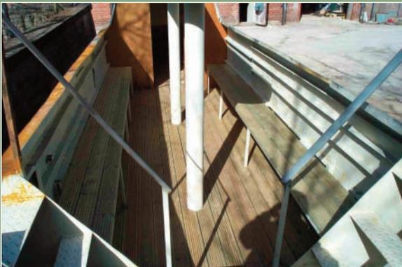
The front deck is covered with garden decking and a plywood sheet is fitted to the back of the forewell.
