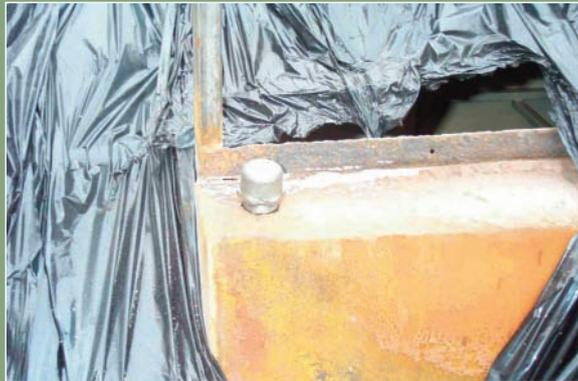
A water filler cap is installed by the front steps. It is not yet linked up though as we haven't put the water tank back in.
