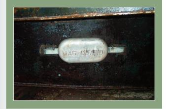
Four brand new anodes are attached below where the water line will be. A grinder is used to remove the paint, dirt etc. from the steel before the anodes are attached (providing a better contact).
