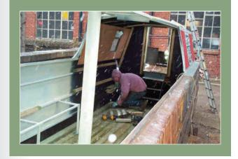
Paul attaches the decking to the floor battens with screws so that more ballast can be added as needed.
