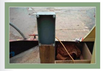
The new control box is fitted to the back deck. The old single lever control stick has been cleaned up and will be used but we have bought new cables. There is no point having to attend a breakdown call for the price of a couple of cables.
