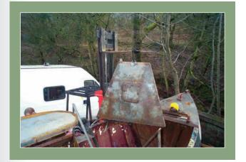
The old water tank is removed so we can clear the mud, water and scale from the bottom of the bilge.
