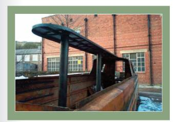
Saturday morning and as ever Paul's up first thing. By the end of the morning he has welded the roof supports in place. He then makes a box section frame to hold the roof. The frame is attached to the supports and then the roof is welded onto the frame. The roof is bent to the same profile as the back cabin with G clamps. Finally the sides are welded onto the finished structure.
